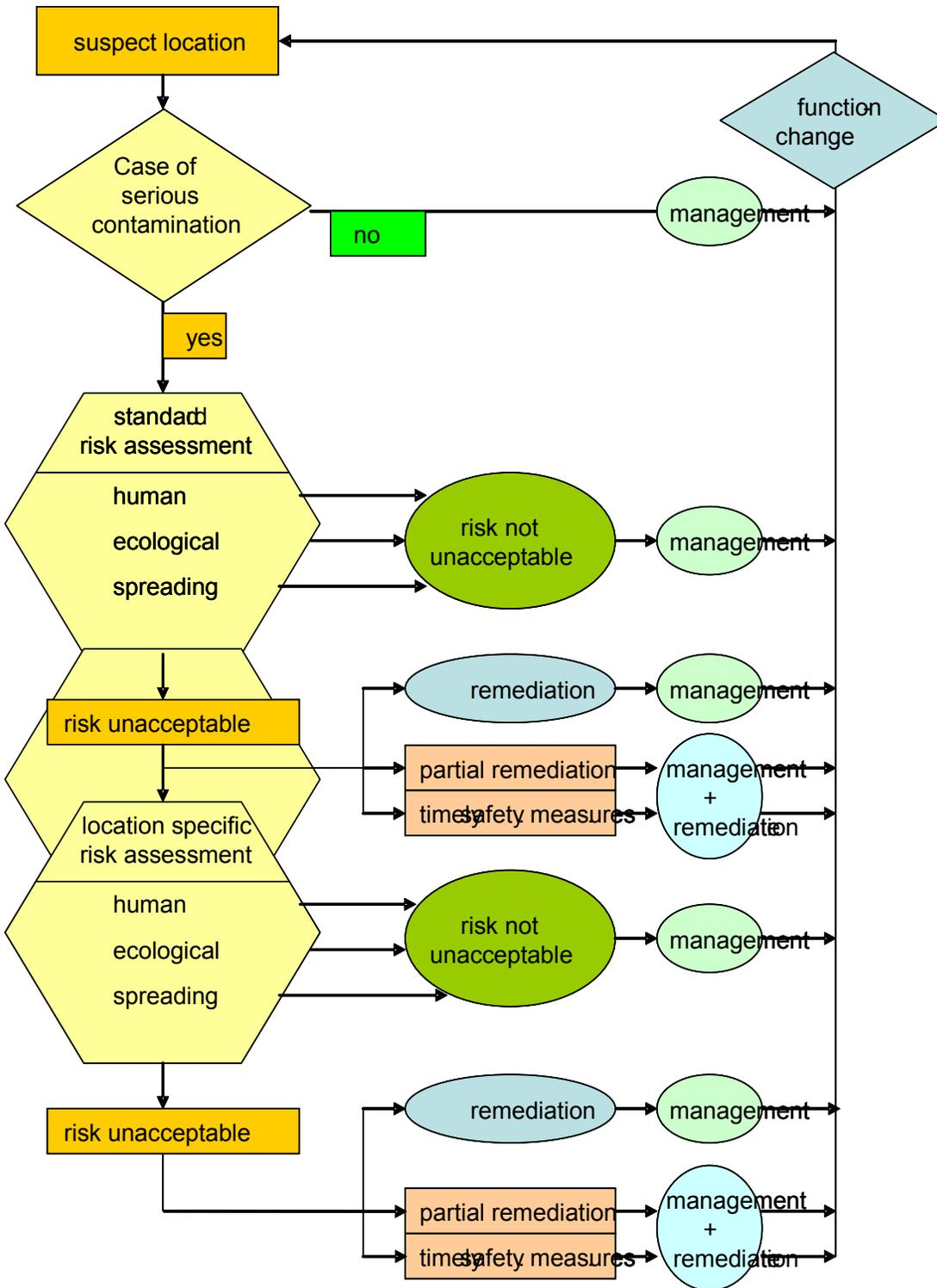
Figure 1: Diagram of soil remediation process
